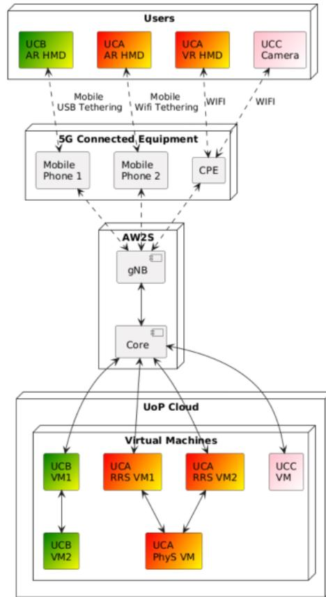
Fig. 2. Component Diagram of all UCs at Patras 5G testbed. Components of the same color correspond to components of the same UC.
